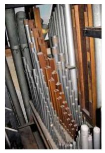
Approaching its centenary it was clear that the organ needed major restoration if it was to remain in use. Critical parts were worn; pipes either didn't work, or worse, sounded when they weren't supposed to because air was leaking between the proper wind channels; everything was covered in 100 years of dust.
